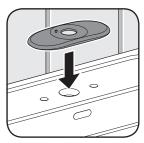
Mount cover plate if required. Plumber's putty is recommended to seal cover plate to the sink. Security pin must be located on the left side.
