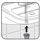
Mount bracket from underneath. Place hoses through large opening and mounting rod through small opening. Make sure flange sits securely against surface.
