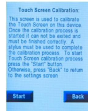
Calibrate screen: Use stylus to tap each screen corner as directed by the screen instructions. (Only required when having difficulty with screen touch response.)
