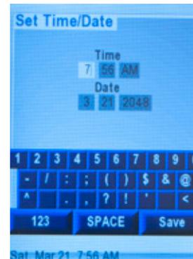
Set time and date: 12 hour clock; MM/DD/YYYY. Must be set after each battery charge.
