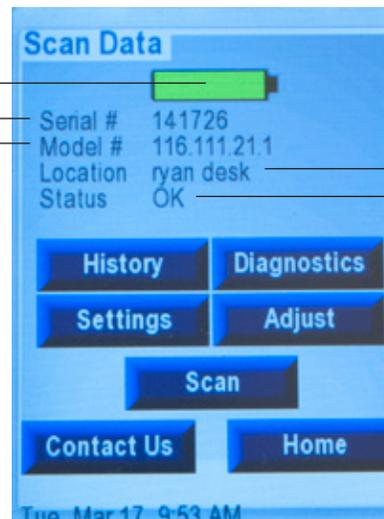
**Location** — Manually entered fitting reference name to assist with locating the fitting in the future. For example, “2nd floor men’s on the right”. Default value is “Not Set”. See Section 2.3 for instructions on how to add or update the location field.
