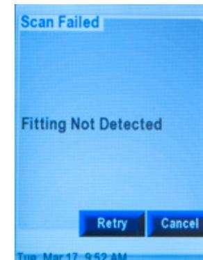
If fitting is not detected within 30 seconds, a SCAN FAILED message is returned. Suggested step, try again, slightly closely to sensor eye
