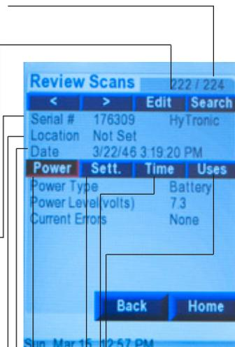
**Uses** — time is use; number of uses, uses/day (calculated) — helps to plan for PM work and calculate water savings.
