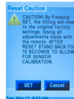
**Warning:** Some data loss may occur when using RESET - (example, but not limited to number of uses, uses per day). This occurs because scan data is not written to the module immediately. The information buffers for a certain time, and is written to the module at some later date. Any scanned information in the buffer will be lost by using RESET.
