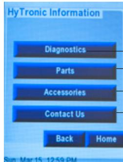
**Diagnostics** — Troubleshoot CFC electronic fittings. Mobile diagnostic tool to directly analyze symptoms and provide fitting specific solution paths. See section 4.2 for more detail.
