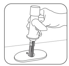
4 Feed supply hoses through faucet mounting bracket. Slide bracket over faucet mounting bolt and secure to sink.
