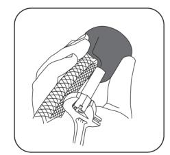
5 Flush lines at supply stops and attach to outlet. Insert filters into ends of each supply line. The blue sticker indicates the cold water supply hose.
