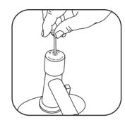
2. Turn the plastic serrated adjustment nut to adjust the timing: counter-clockwise to shorten time, clockwise to lengthen time.
