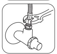
6 Install Outlet - Using outlet key, turn outlet clockwise until tight.
