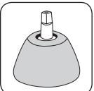
eons over handle stems. Handles should cover the sealing washers.3
