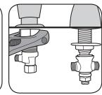
7. Using adjustable wrench, tighten underbody nuts.
