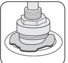
3. Place a sealing washer 4. Insert retaining clips firmly into channel on each valve body. Remove hanger from spout hole.
