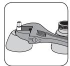
8. Using adjustable wrench, tighten. handle holddown of nuts.
