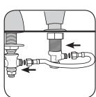
11. Connect right supply line to right handle and right side of water connector.
