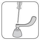
9. Align both handles on stem as desired. Insert index 👺 buttons, screws, and tighten.
