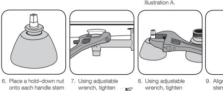
onto each handle stem and hand tighten. underbody nuts.
