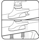
4. Remove outlet and flush lines.
